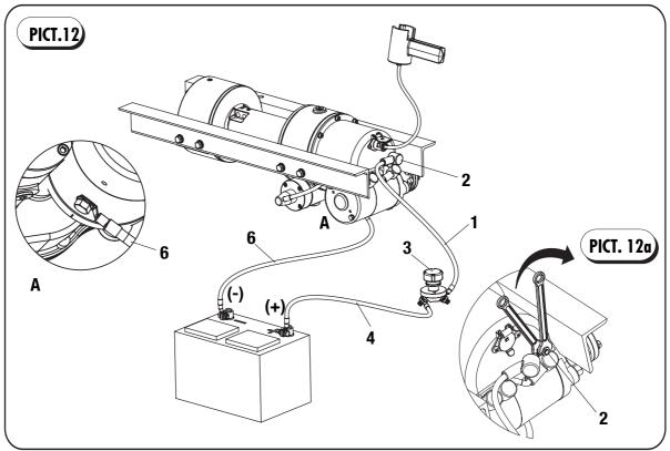
Connect cable (1), length (1,5 Mt), from power supply terminal (2) to battery switch terminal (3). Connect cable (4), length (0,5 Mt), from battery switch terminal (3) to positive battery terminal. Attach ground wire from motor housing (capscrew 3/8") to negative battery terminal (detail A, pict.12).
